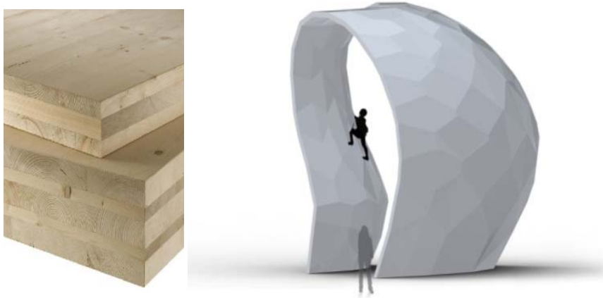
Figure 1. left : Standard Cross Laminated Timber (CLT) panels (image: www.finnfinnholz.com ), right : Irregular structure with flat panels of CLT
